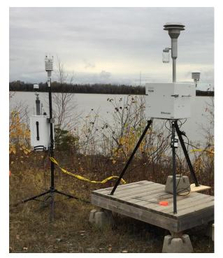
Figure 4: PQ200 and Aeroqual Monitor
